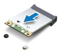
CAUTION: When the Mini-Card is not in the computer, store it in protective antistatic packaging. For more information, see "Protecting Against Electrostatic Discharge" in the safety information that shipped with your computer.
